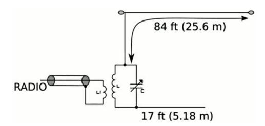
If you're at a site calling for an end-fed antenna, the W3EDP may be the one for you. Rather than run the short wire off in an odd direction, slightly better performance results from configuring the two wires to produce an end-fed Zepp.
