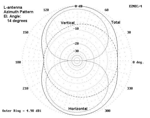
Notice that the vertically polarized circle of radiation is slightly offset from being truly symmetrical around the antenna. That shift is due to the presence of the horizontal leg. The horizontally polarized radiation shows the typical dipole figure-8 pattern, but not as strong as it would be if both halves of the antenna were horizontal.
