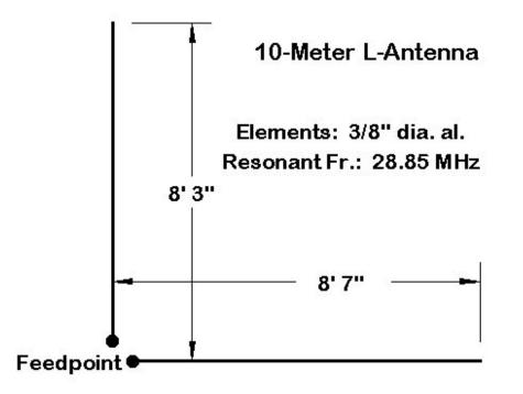
What has happened is that the rotated Vee and the 1-legged vertical have turned into the same antenna, which is simply the L-Antenna. Figure 1 shows a sketch of how to build one from 3/8" diameter aluminum tubing. I claim no originality for the antenna, since a version of it has appeared in Moxon's *Antennas for All Locations*. Apparently, the first commercial version appeared in the 1950s.
