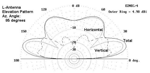
Figure 3 shows the elevation pattern of the antenna, again at 30 feet up. The pattern is taken through the axis of maximum gain, which is--for the total field--about 5 degrees off a true perpendicular line drawn to the horizontal element.
