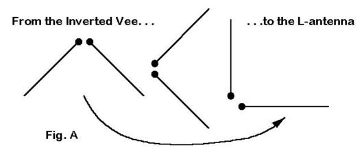
First, consider the common inverted Vee, shown in Figure A. When the legs make a 45-degree angle with the landscape or with a vertical line drawn between them, the impedance drops from the usual dipole value of 70 Ohms to about 50 Ohms.
