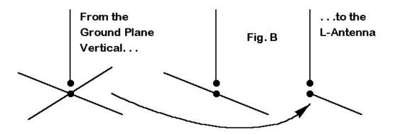
Let's try that again, but this time, begin with a 1/4 wavelength ground plane vertical with the base at the 30' mark, as shown in Figure B. This vertical antenna is actually a special type of dipole, one where one of the legs consists of 4 wires arranged symmetrically and at right angles to the vertical part.
