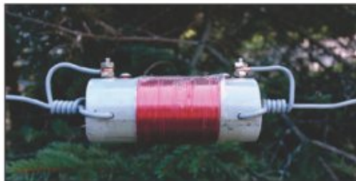
The DX-EE uses inductive loading on the 40/20 meter wires to reduce the overall length to just 40 feet.
