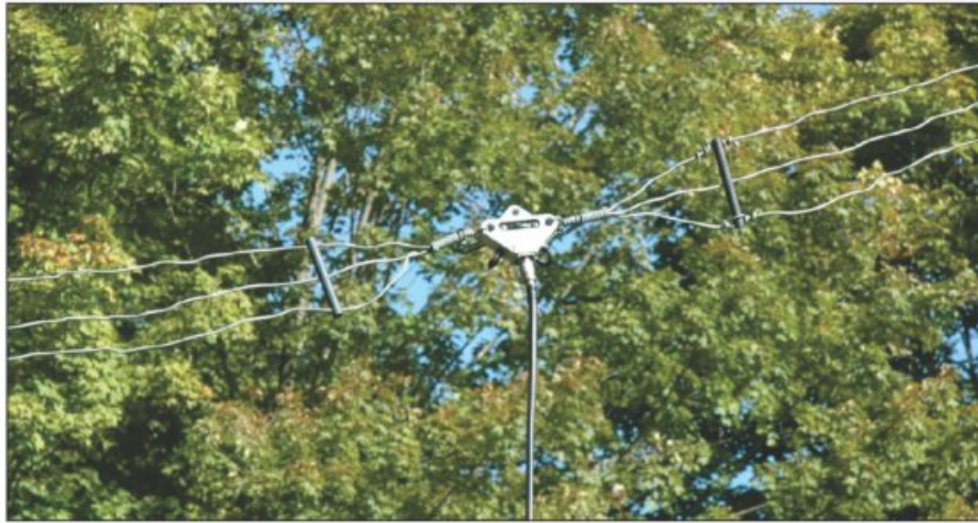
The center section of the DX-EE at a height of 25 feet.
