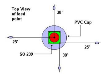
NVIS Tri-Band Antenna for 75, 60, & 40 Meters
