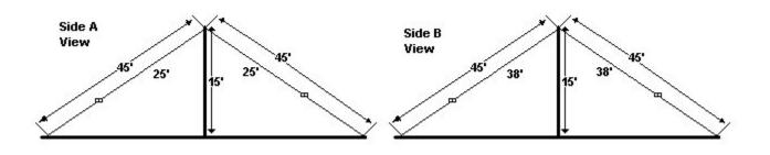
Dr. Jelinek used two sections of 1 1/2-inch PVC pipe for a mast. If you have the room to install this type antenna, it may very well be the ideal antenna for Regional MARS communications.
