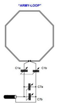
Basic tuning and matching circuitry employs two high voltage twin gang 468pF variable air-spaced capacitors. An extra 450pF was switched across C1a and C1b to cover the entire 2-5MHz frequency range for coarse tuning. For improved fine tuning, capacitors C2a and C2b were provided with a 12-way switch to select one of twelve high grade mica capacitors (750-8250 pF) for additional impedance matching.
