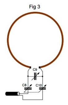
Even though the four diagrams above show single variable capacitors, high power loops often use two series variable capacitors to double the voltage rating and avoid flashover between the capacitor plates. Even at modest QRP power levels voltages in excess of 1000 volts can be present across the tuning capacitor and matching capacitor.
