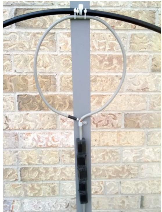
Ferrite beads attached to coupling loop for suppressing common mode currents
