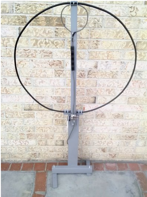
Magnetic loop mounted on 55-inch wood stand.
