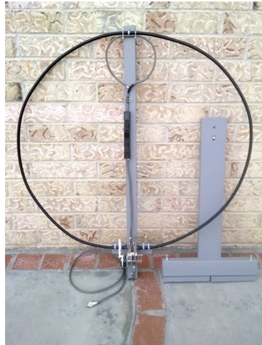
Magnetic loop with wood stand disassembled.
