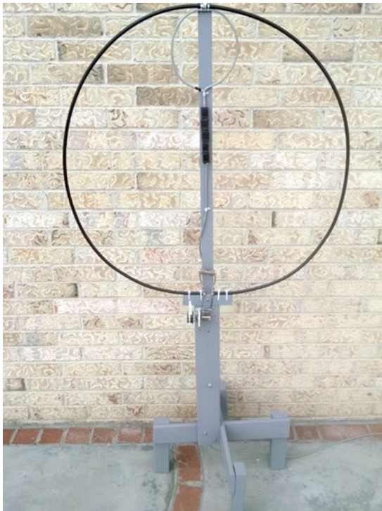
Magnetic loop mounted on 67-inch wood stand
