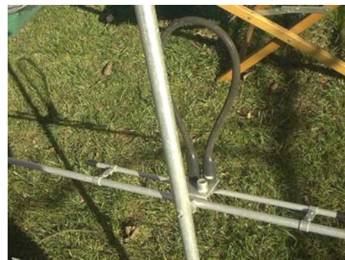
Fig 32 – A Half-Wave Balun
